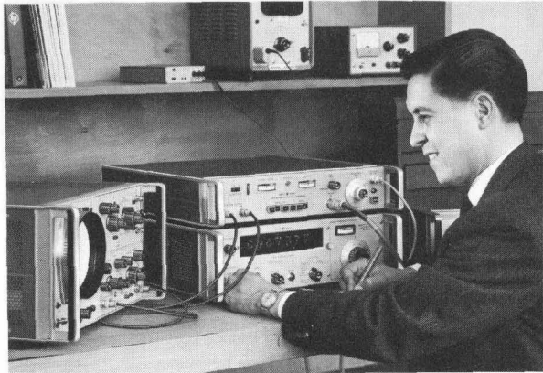
Fig. 6. Microwave Frequency Converter phase-locks built-in transfer oscillator to sub-multiple of microwave input frequency. Counter reads transfer oscillator frequency with characteristic precision. Converter permits measurement of frequencies of CW, FM, AM, and pulsed RF signals.
